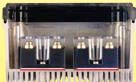
Installation example of solid state relays in an aluminum Ultimheat housing (thermal compound in red).
